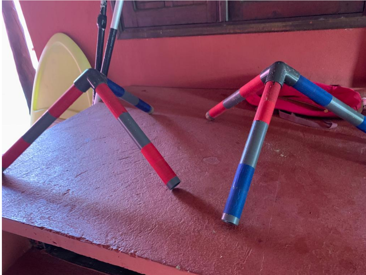
Fig. 3: Metric reference build out of PCR tubes and filled with sand.
